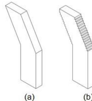
Fig 1. Stair-casing Effect on Build of Part (a) CAD model of actual part and the (b) Component fabricated using AM
