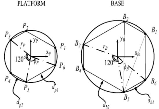
Fig 4. The SRSGP with Design Variables and Constraints
