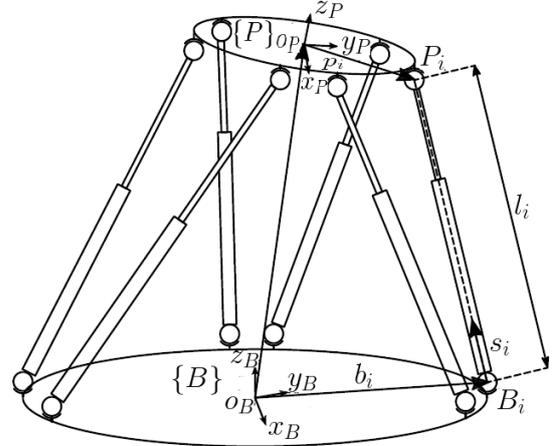
Fig 3. Schematic Diagram of a SGP
