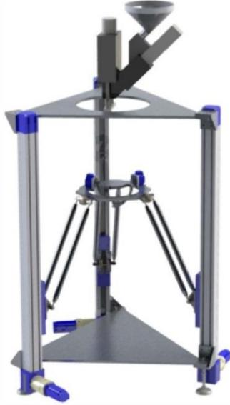
Fig 2. Delta Manipulator for Metal Injection Moulding [5]
