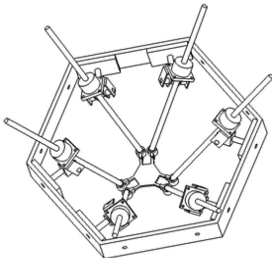
Fig 5. Schematic Diagram of SRSGP for AM
